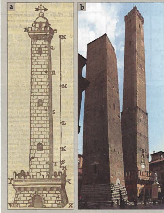
Figure 3. The Asinelli Tower, which Giovanni Riccioli considered to be “as commodious as possible” to falling-body experiments, stands nearly 100 m above the heart of Bologna, Italy. (a) Riccioli’s sketch illustrates his experimental findings: A ball dropped from the tower’s summit, point O, reaches points C, Q, R, S, and T in times corresponding to 5, 10, 15, 20, and 25 pendulum strokes, respectively. (Image from ref. 14.) (b) A photo shows the tower as seen today.
