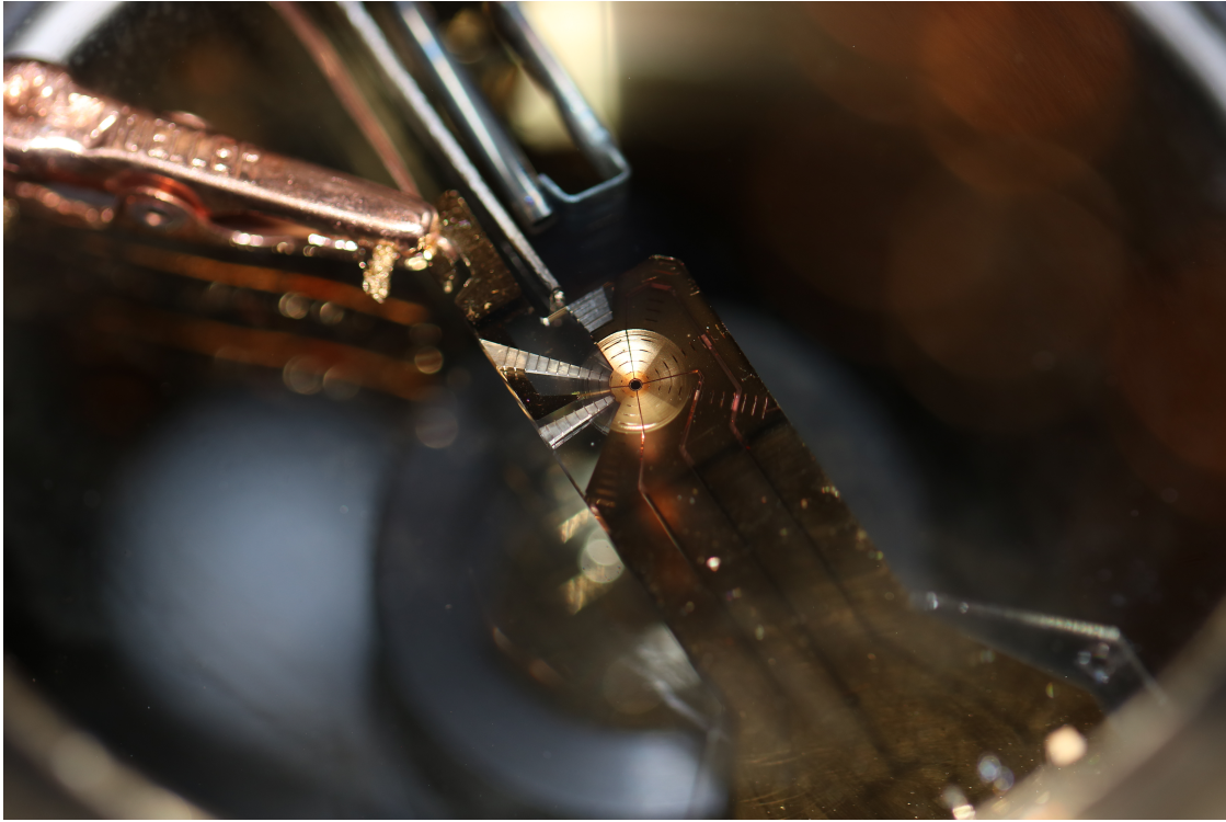
Figure 2.2: Camera image of the oblate ring trap. The trap has a total of 8 pie-slice shaped DC compensation electrodes (4 above, and 4 below the trap), and RF is delivered to the central ring. Tapered trenches were used to couple light to the trap, and imaging was done from above and below.
